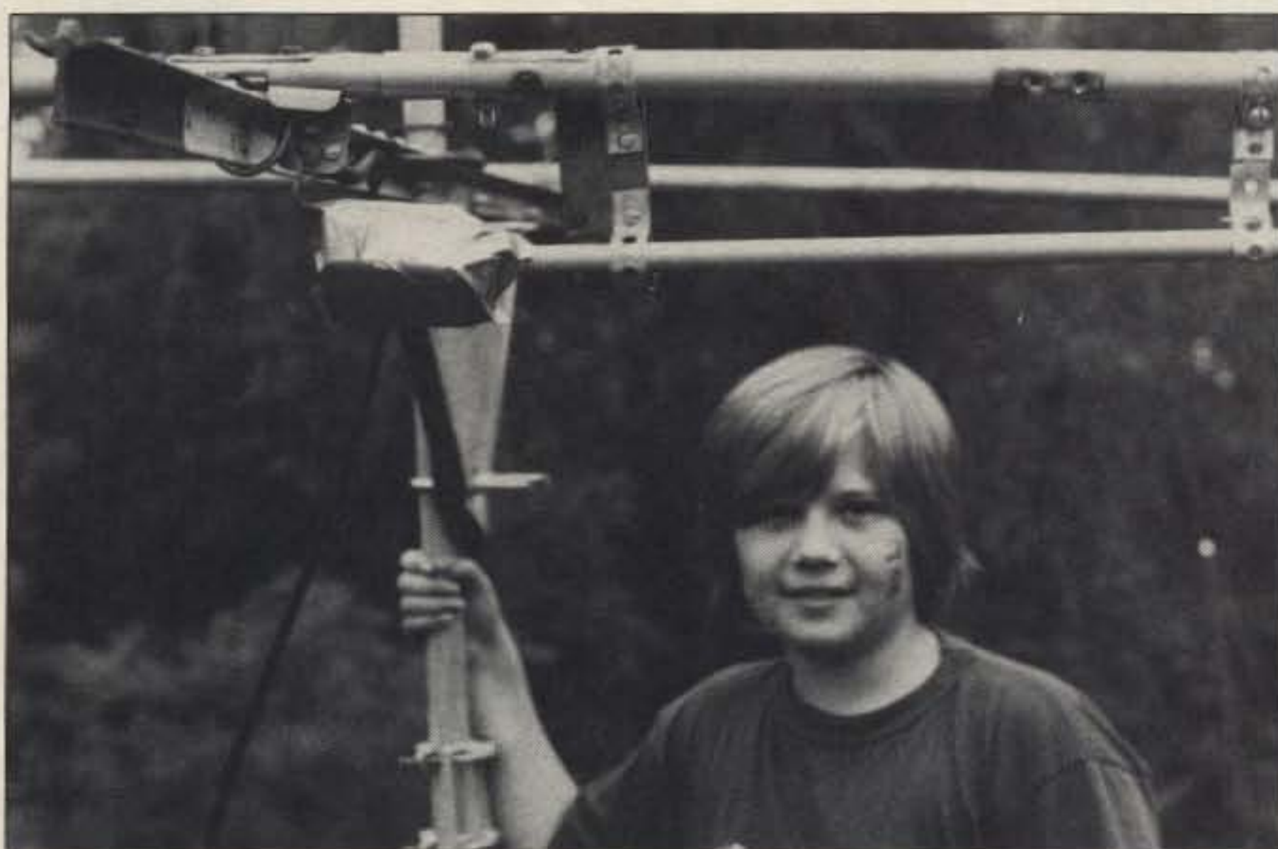
Photo B. Close-up of the Gamma match and the organic rotator. The variable capacitor has been covered with a plastic bottle and tape.
